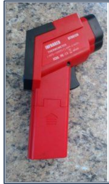
DT8000 (-50°C to 1200°C) Accuracy: \pm 2\% or 2°C Distance Spot Ratio 16:1
