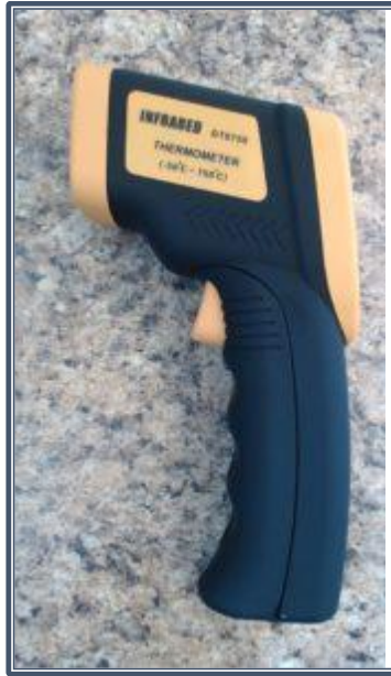
DT8750 (-50°C to 750°C) Accuracy: \pm 2\% or 2°C Distance Spot Ratio 12:1
